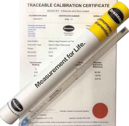
Following of the ban on specification mercury laboratory thermometers in October 2017, S.Brannan & Sons has developed a range of spirit filled, high precision thermometers. These thermometers are supplied complete with a traceable calibration certificate and are presented in a sturdy cardboard cylinder for storage. The thermometers are made to the highest possible standards and are checked at every stage of manufacture to the requirements of our ISO 9001
