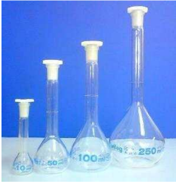
1621A Volumetric flasks with One graduation mark with glass/PE stopper ISO1042, DIN12664
